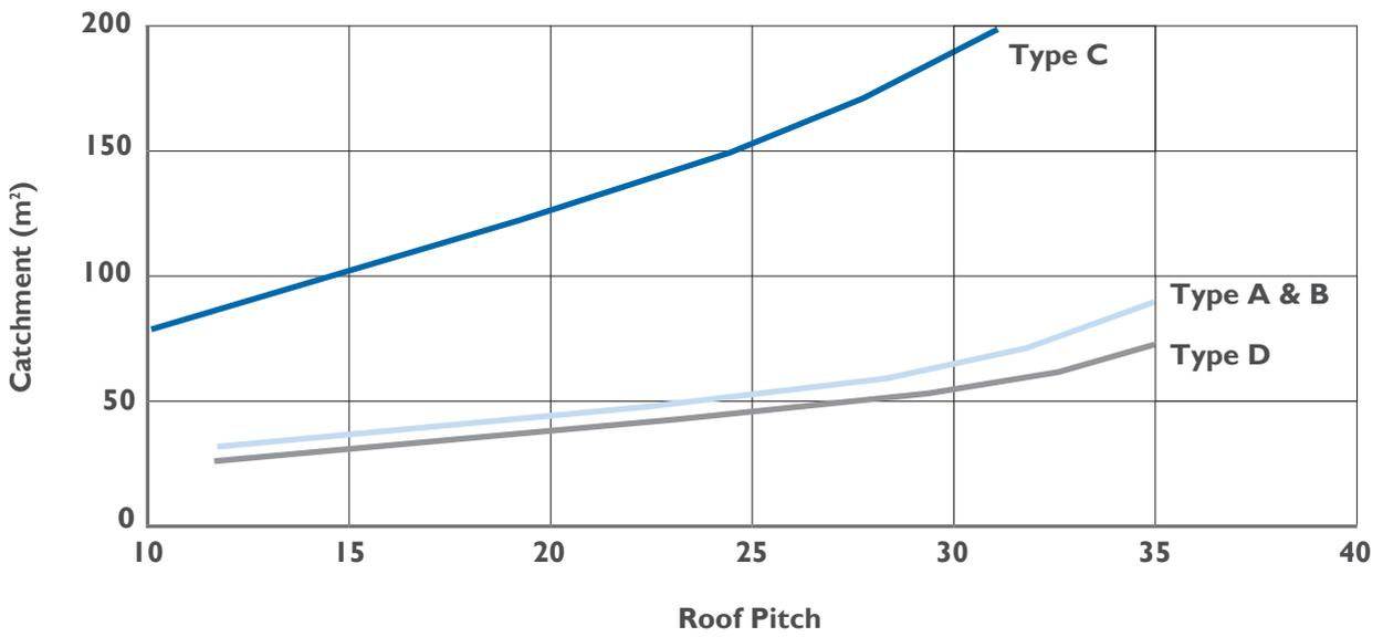
Note: A & B capabilities only equal if hook section A has 20mm height
