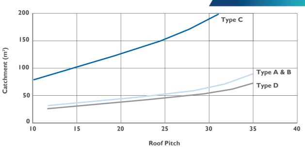
Note: A & B capabilities only equal if hook section A has 20mm height Type C recommended when roof pitch is <12°
