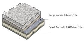
Roofs coating systems allow the natural reactions of the galvanic coatings to occur without effecting the protection offered to cut edges or scratches.
