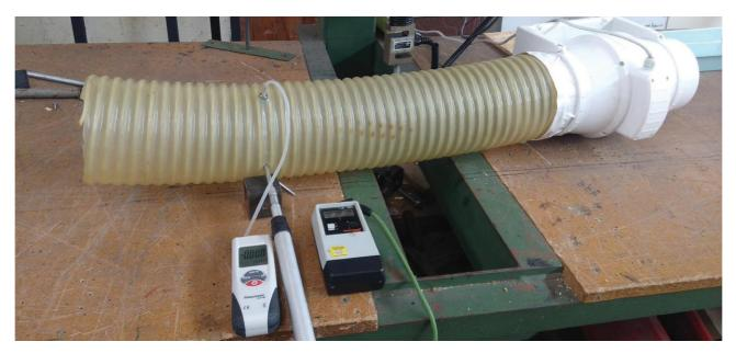
Ducting, fan, manometer and anemometer
