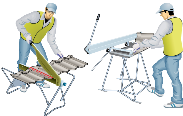
Figure 14.7.4.2 Gable end tile being cut then bent
