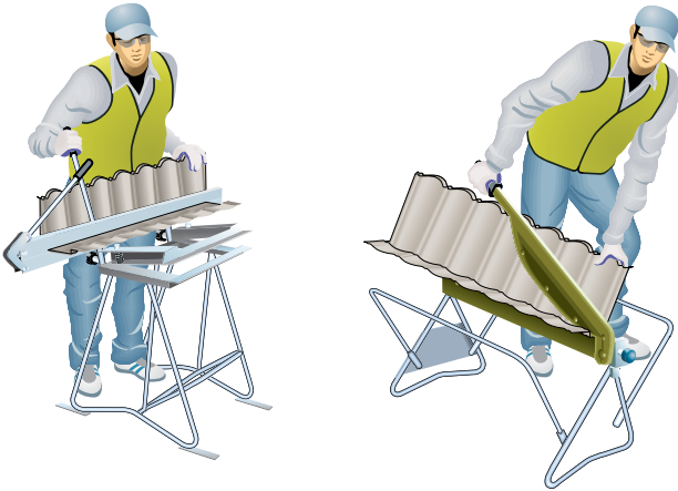
Figure 14.7.6.3 Ridge tile being bent then cut
