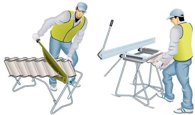
Figure 6.2.7.2 Valley tile being cut then bent
