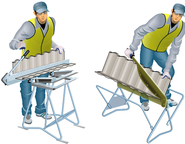
Figure 6.2.6.3 Ridge tile being bent then cut
