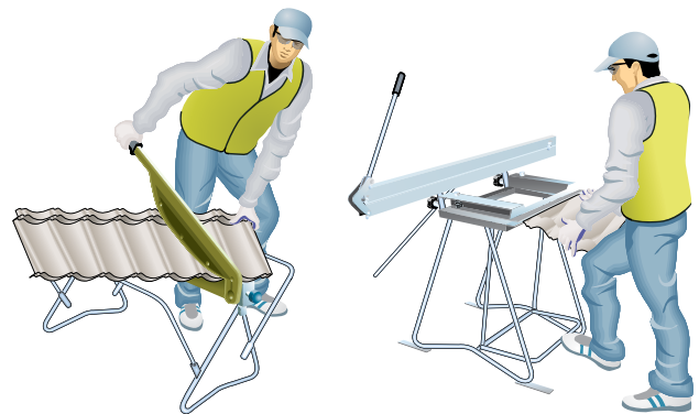
Figure 14.7.7.2 Valley tile being cut then bent
