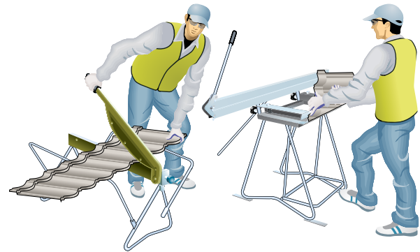
Figure 14.7.5.2 Cutting and bending a hip tile
