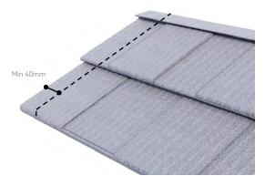
Cut the fold of the panel's nose, cutting the underside only, then snip the head fold partway through.
