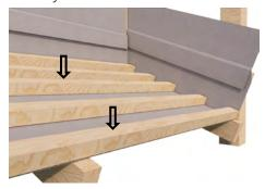
Install CF Shake or CF Shingle panels up the roof, starting at the eaves. When a wall is met, create an upstand of at least 40mm.
