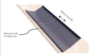
Install CF Shake or CF Shingle panels up the roof, starting at the eaves. When the valley is reached, turn down the sides of the panel into the valley, ensuring a minimum of 50mm space between the panels on opposing sides of the valley. The cut edges of the turn down should have a minimum clearance of 20mm and must not touch the valley.
