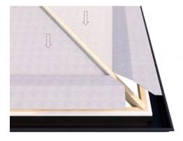
Underlay should be draped over the top of the already-installed batten/s at the eaves.
