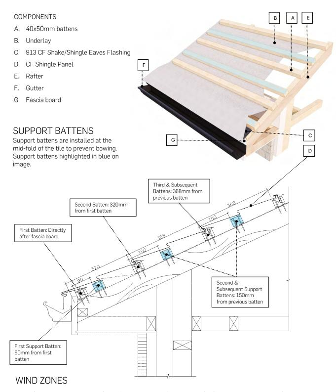
When fixed in accordance with Gerard's systems specifications, the CF Shingle panel is suitable for use in all NZS 3604 wind zones, up to and including Extra High. In NZS 3604 Very High building wind zones, 150x25mm battens are to be secured using 2x90x3.15 power driven nails for the main and periphery roof areas. For Extra High Wind Zones 10g self–drilling screws (80mm long) must be used to fix battens to trusses.
