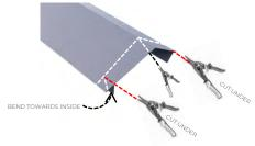
Fold the top down, overlapping the centre point to create a clean front.
