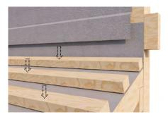
Install CF Shake or CF Shingle panels up the roof, starting at the eaves. When a head wall is met, create an upstand of at least 40mm at the head of the panel.
