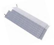
Hook the next trim into the installed trim's head and fasten, making your way up the hip.
