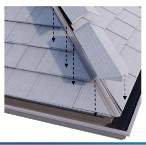
Take care to fasten at the outside edge of the tabs to avoid penetrating the weather channels of the under channel.
