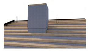
Install CF Shake or CF Shingle panels across the roof, starting at the eaves. At the penetration, turn up the panels by a minimum of 40mm on all sides.
