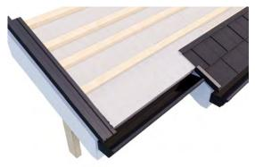
Measure and cut the head off the first course of panels at the short edge of the roof. The head should align with the head of the alreadyinstalled panels. Hook the nose over the eaves flashing and fasten in place.
