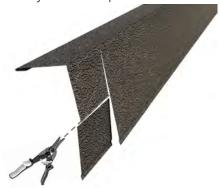
Fold in the flap slightly and fold the front down creating a box-end.
