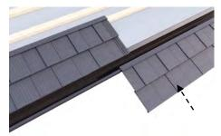
After installing the first course, fit the second course by hooking the nose of the second course panel into the rear head check. Stagger the panels to give an irregular pattern across the roof.
