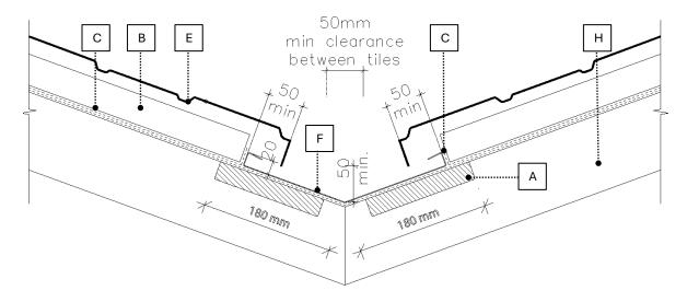
Note: Valley trays are held in place with a clip or nail bent over the top of the valley. Do not nail inside the valley.
