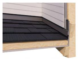
Once side flashings are installed, the builders can install the wall cladding.
