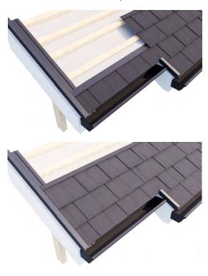
Install the rest of the panels and then finish with the barge cover and ridge trims.
