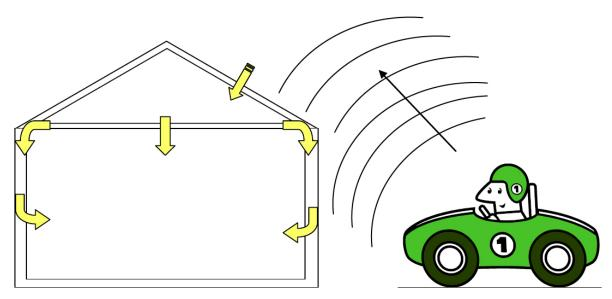
Figure 1: Flanking transmission paths from the roof.
