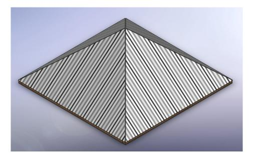
Figure 2: Test roof system for laboratory measurements.
