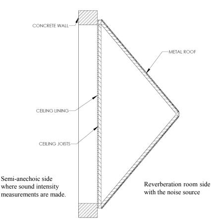
Figure 3: Simplified cross section of test roof system mounted to the concrete wall of the reverberation room. The trusses of the roof are not shown.
