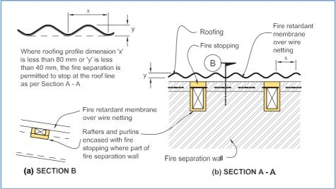
Figure 4.2 and 4.3; Junctions of fire separation - 1 and 2
